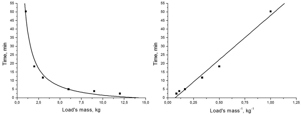
**Figure 2. Plot of cutting time subject to loads mass for the nichrome wire (d=0.4 mm), and it's linearization. Fitted by hyperbola.**
