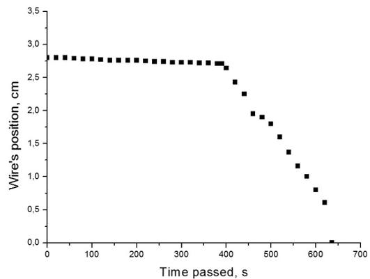
**Figure 4. At first wire moves slow, as it's only accumulating heat, required for melting first portion of ice. But then cycle finally starts, and wire moves with constant velocity.**
