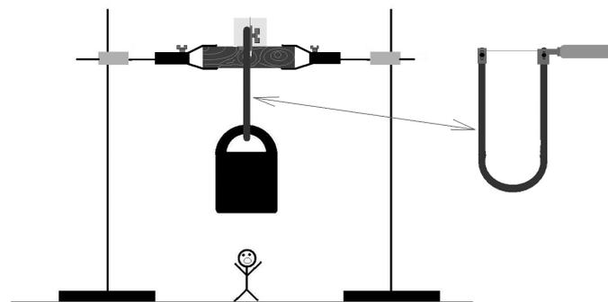
**Figure 1. Experimental setup. After wire exits ice, it falls onto the wooden block and tears apart because of the impact. Too bad for the small human...**
