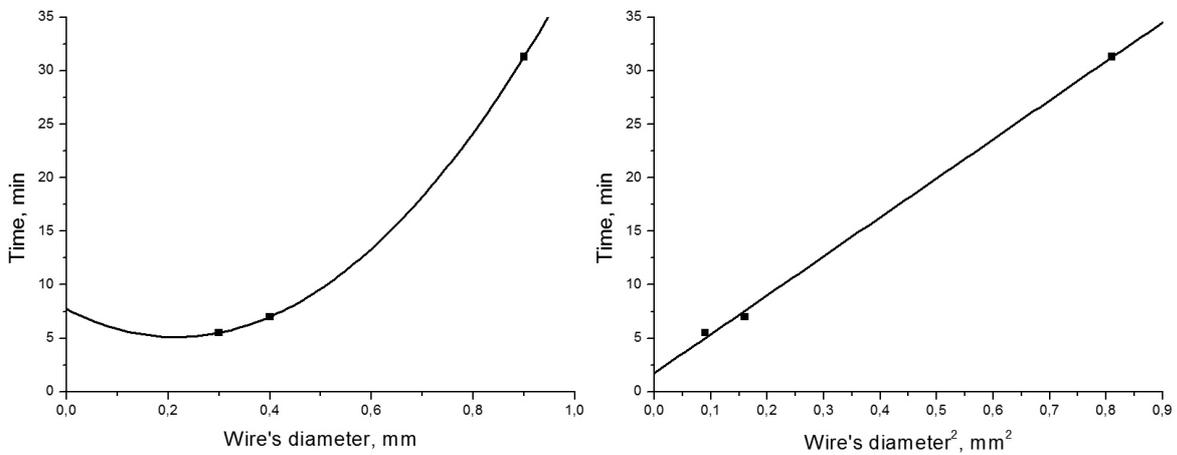
**Figure 3. Time of cutting for three nichrome wires with 6 kg weight attached, and linearization of this dependence. Fitted by square parabola.**
