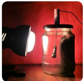
This amazing phenomenon is an example of so called photoacoustic effect when light results in an acoustic wave. The effect is easy to produce, but a serious explanation will be a tricky task for the IYPT participants. When the light bulb is powered by a 50 Hz AC current, the resulting sound has the dominant peak at 100 Hz, audible as a constant, low hum or buzz.
