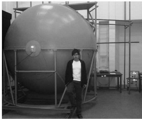
Figure 5: the integral sphere used in the illumination experiments, at University of Tehran
